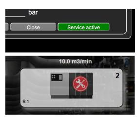
The grey "Activate Service" button changes to "Service active" and turns green. Another click on this button ends the maintenance mode and the compressor can be immediately reselected by the Airleader.
