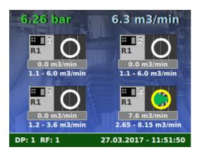
The display of the EASY control shows the current states of the compressors, for VSD compressors additionally the variable delivery quantity, as well as the network pressure and the current total consumption.
