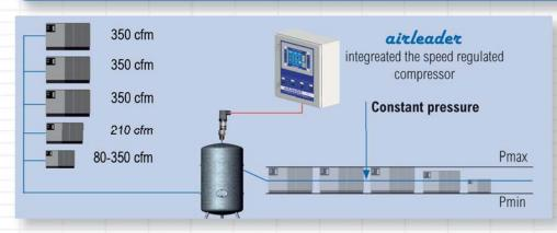
The control strategy auomatically ensures that, compressors connect or disconnect step less within the pressure band. An exceptionally low switching frequency protects the compressors and prolongs their service life.
